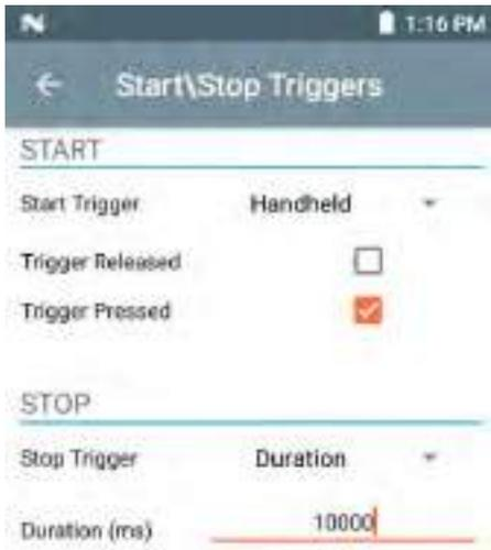
Required input for Start/Stop Trigger settings are as follows:
