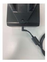
2. Insert the power supply cable into the switching power supply and EU plug into a socket
