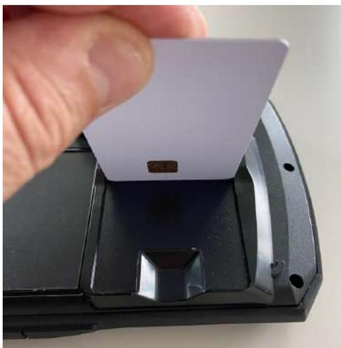
2. Slide the card completely into the reader.
